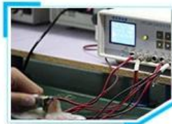
7. PCB board function testing
